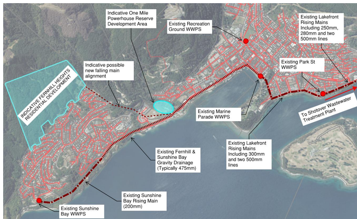
Figure 7: General Arrangement of existing Fernhill and Sunshine Bay Wastewater drainage and Whakatipu Lakefront Mains
