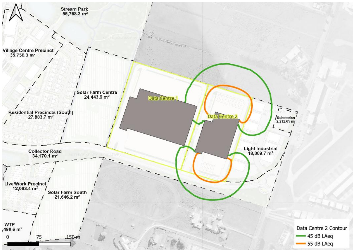
Figure 13 Data Centre 2 noise contour
