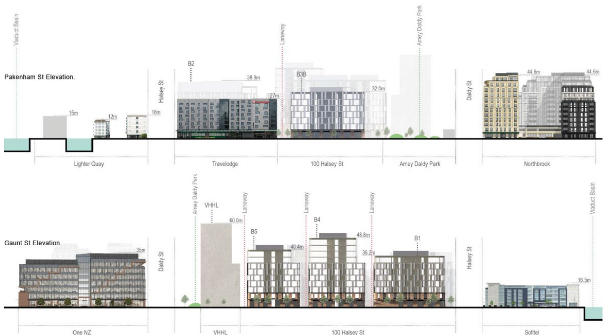
Figure 4.3 Street elevations showing proposed height in context
