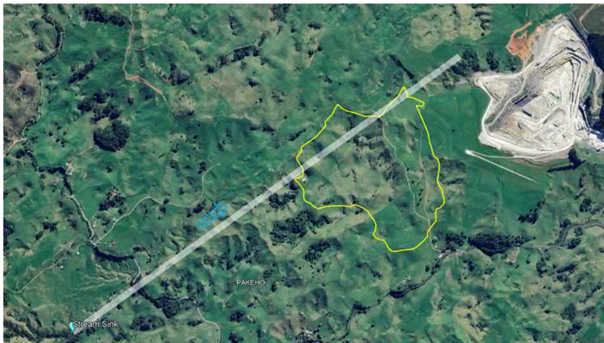
Figure 7-1: Primary North-East structural [thick white line] trend from Stream Sink towards the proposed Southwestern Pit
