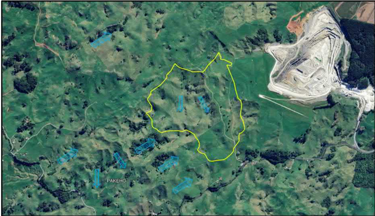
Figure 5-2: Geomorphology of the Southwestern Pit Area [footprint in yellow]. Blue arrows delineate trends in doline and blind gully development.
