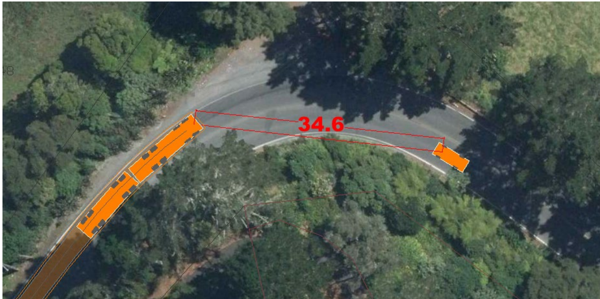
Figure 1: Stopping Sight Distance Assessment
