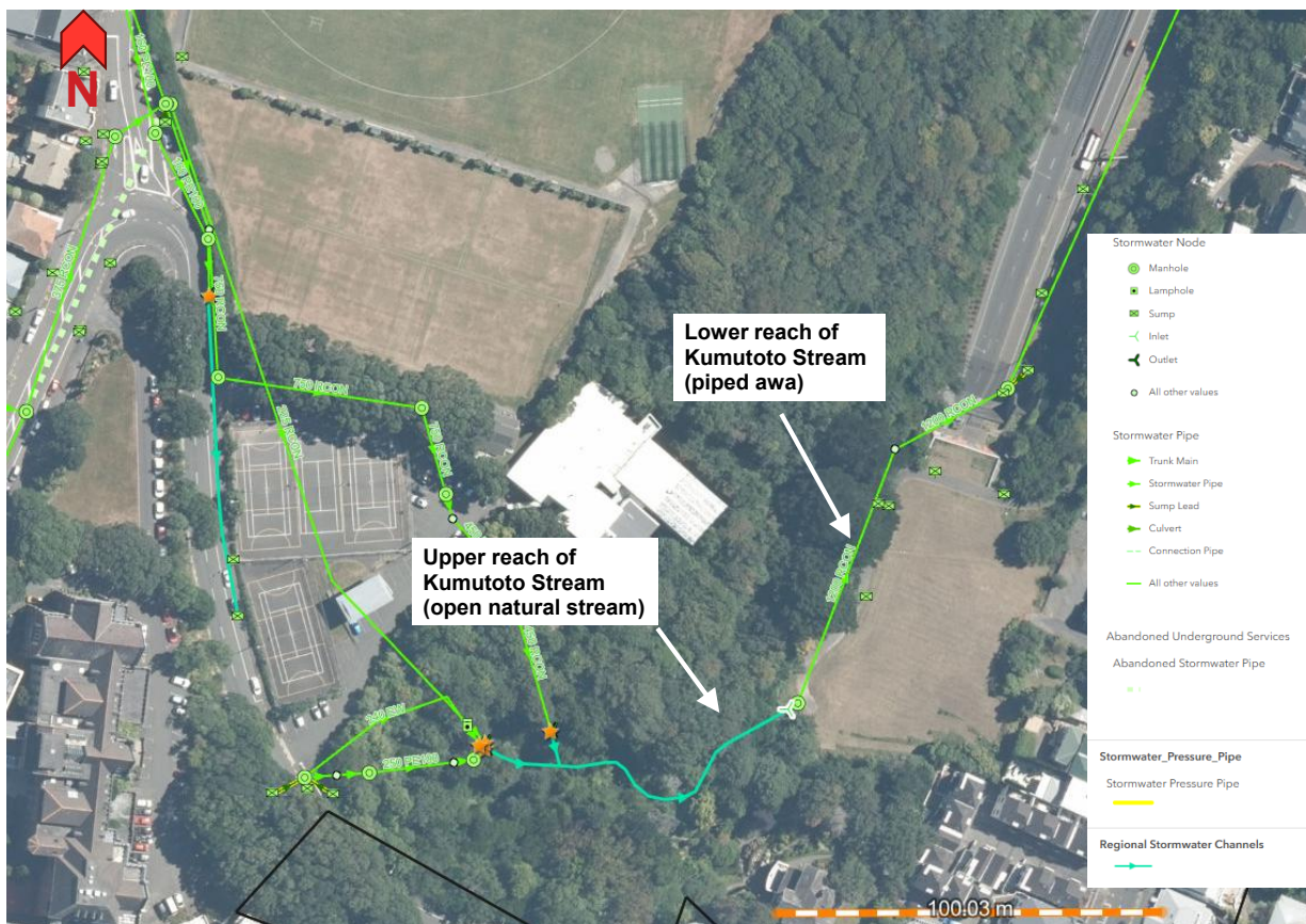
Figure 15 - Kumutoto Stream and stormwater network near northern Terrace Tunnel portal
