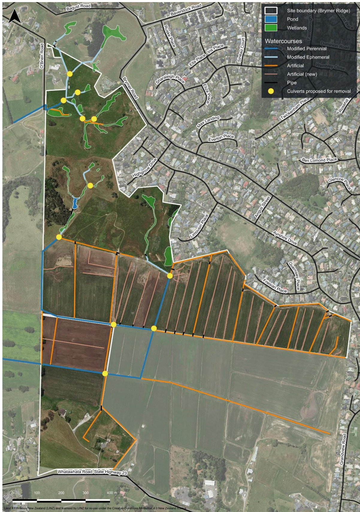
Figure 25: Culverts proposed for removal.
