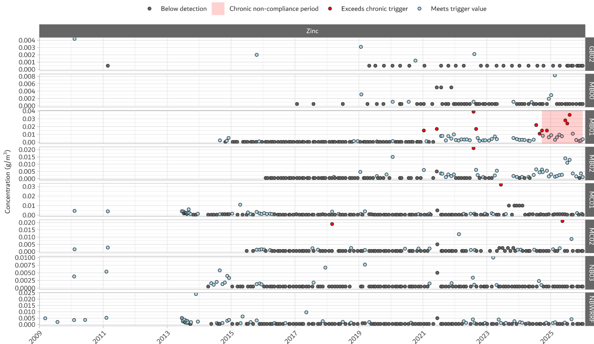
Figure B23. Historical dissolved zinc measurements at key compliance sites within the Waikouaiti and Taieri River catchments, assessed against the proposed triggers.
