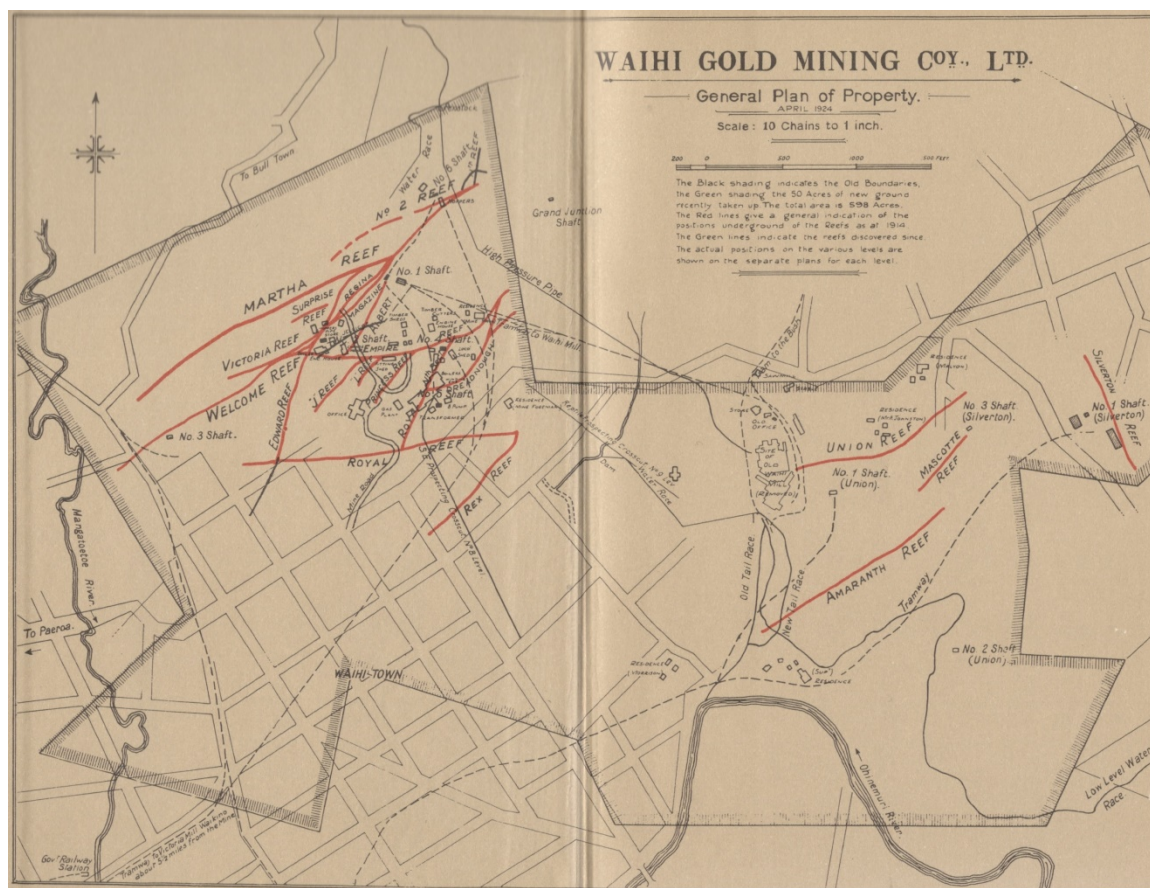
Figure 31. General property plan of the Waihi Gold Mining Company, dated 1924, showing the various reefs, workings, tramways and water races across the Waihi central area (source: McAra 1988: np)
