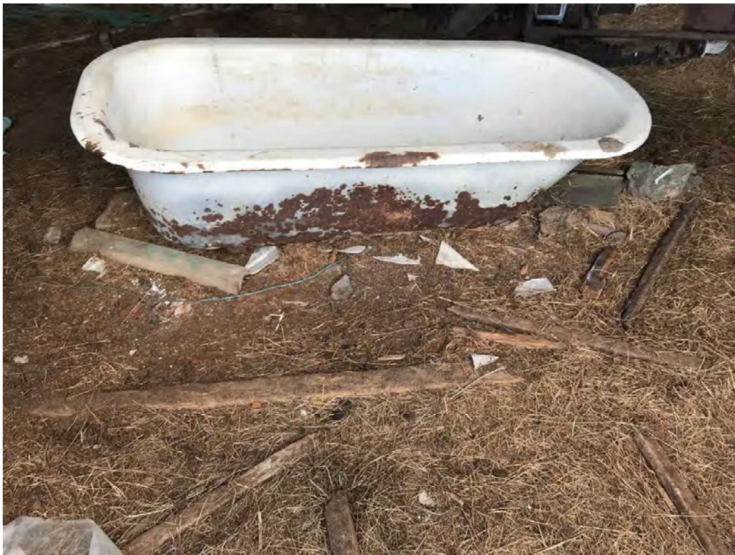
Photograph 8: Interior of the shearing shed with PACM fragments observed on the ground.
