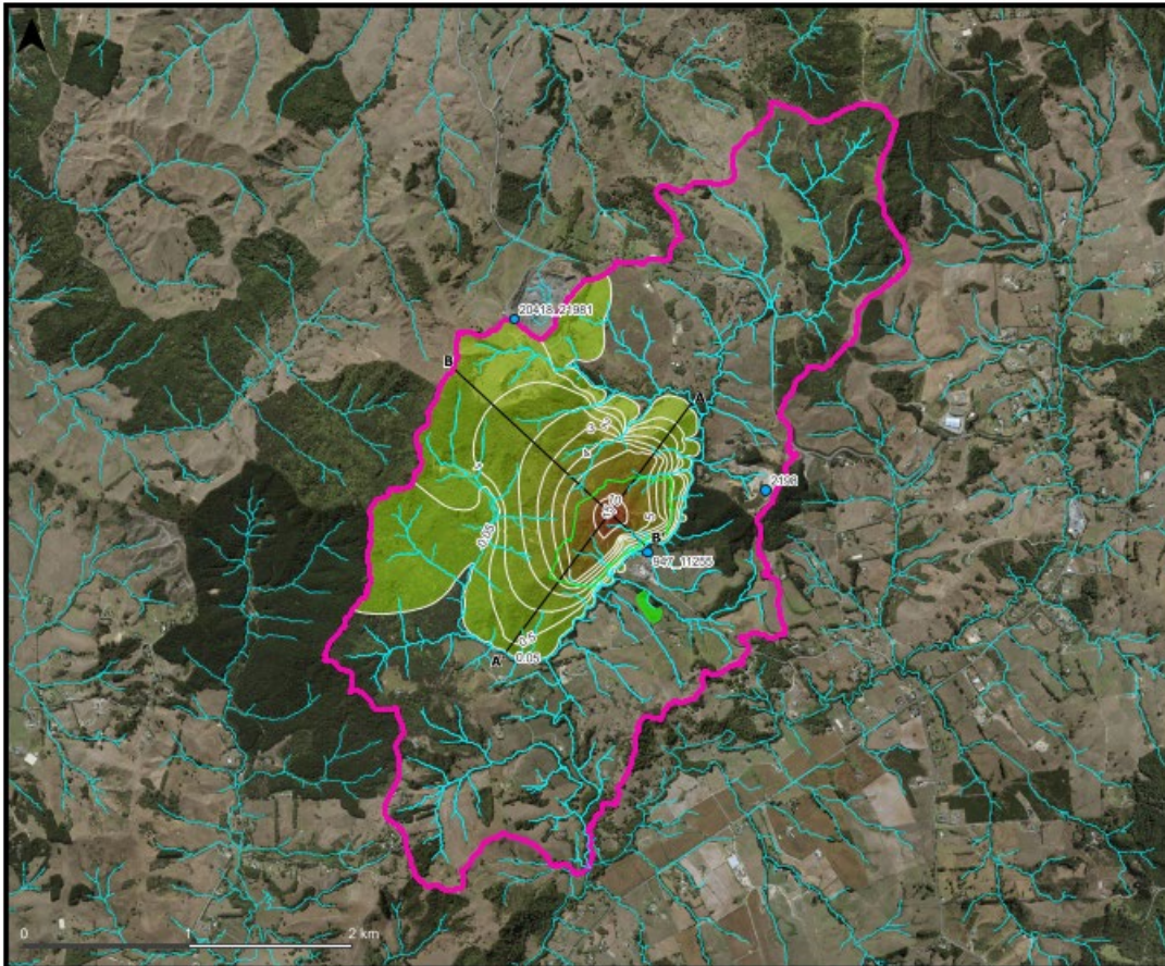
Figure 2: Plan showing the groundwater drawdown contours (Source: FTR, WWLA, March 2025)
