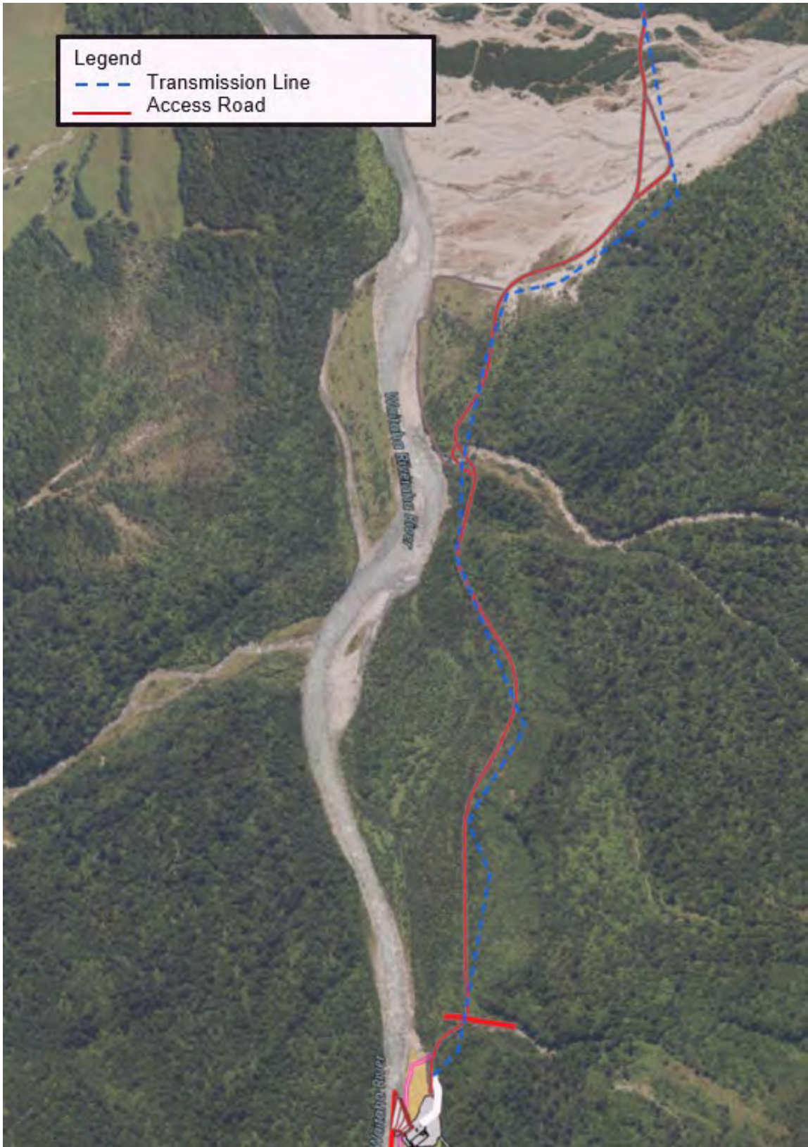
Figure 13: Indicative Alignment of Access Road and Transmission Lines Between McGregor Creek and the Power Station Site
