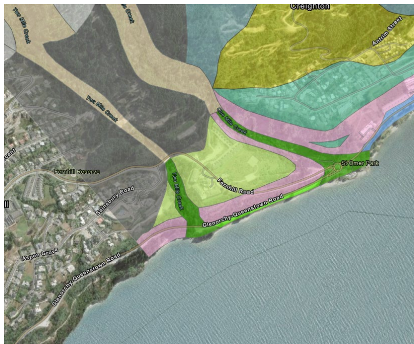
Figure 5: Geomorphic mapping in the One and Two Mile Creek area (Barrell et al, 2009). The areas mapped as 'fan recently active' (dark green) may be exposed to flooding hazards.
