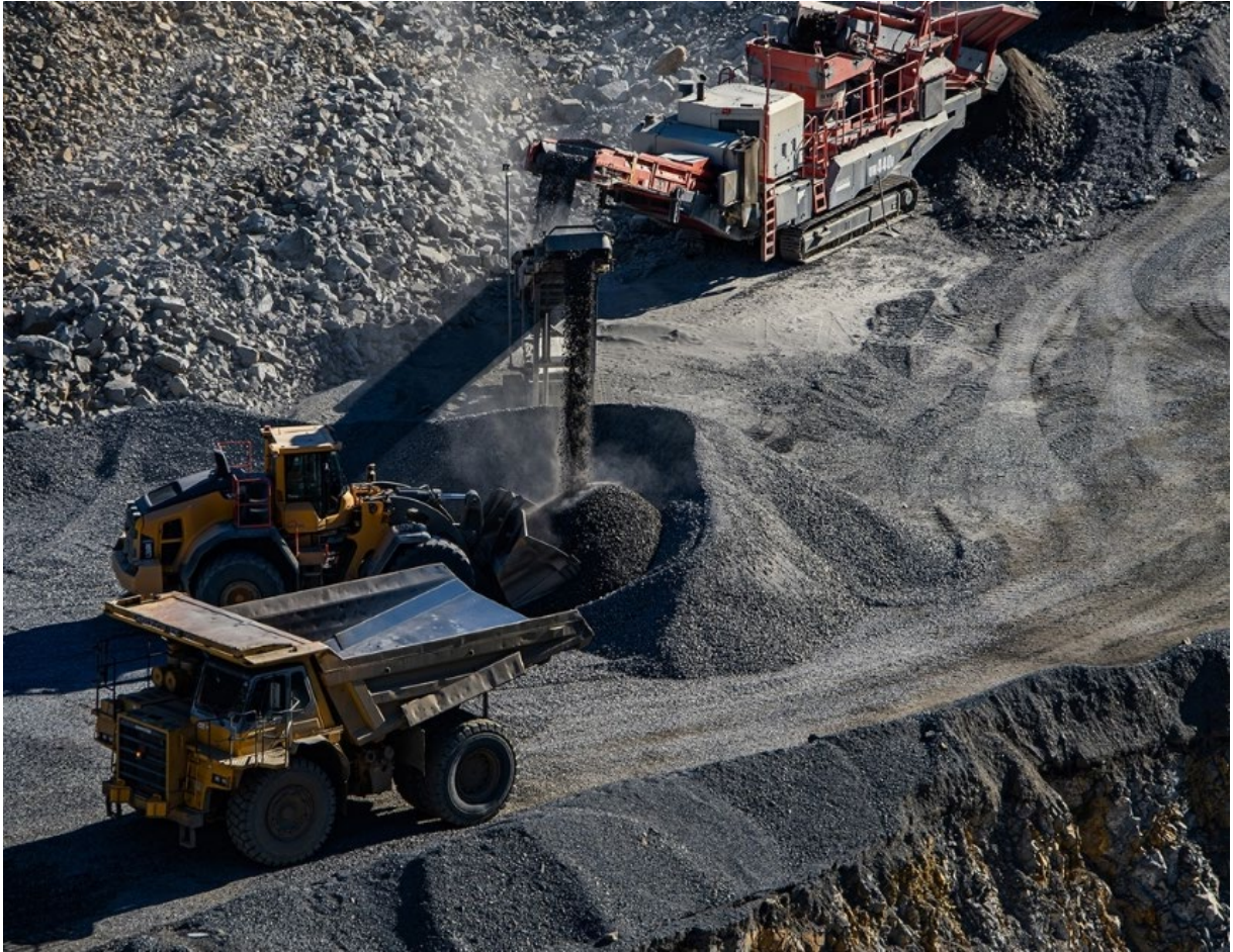
Photo 6: Mobile crushing plant which has the potential to generate dust.
