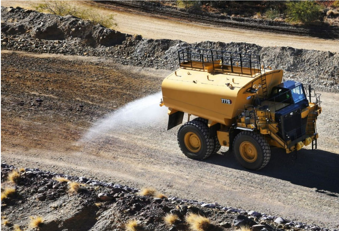
Photo 3: Water cart spraying haul roads.
