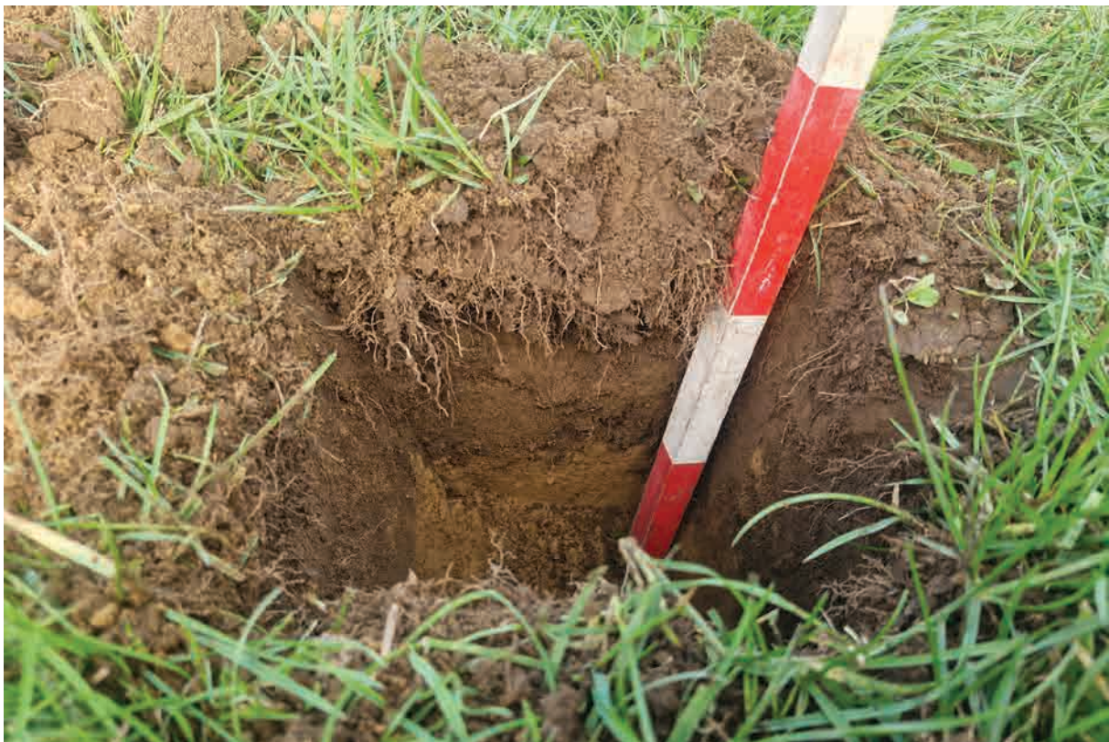
Figure 11. Test pit, scale units are 100 mm.
