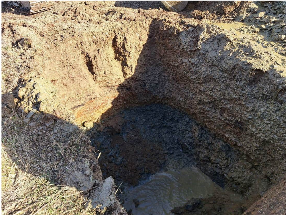
Coarse silty sand overlying coarse medium gravel (Alluvial deposits) within valley floor.
