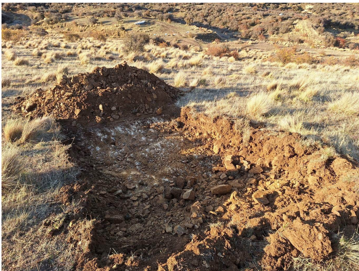
Weathered TZ3 schist with very thin overlying colluvium deposits
