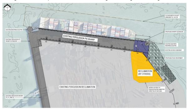
Figure 4 Fergusson FN Eastern Wharf Extension - Plan
