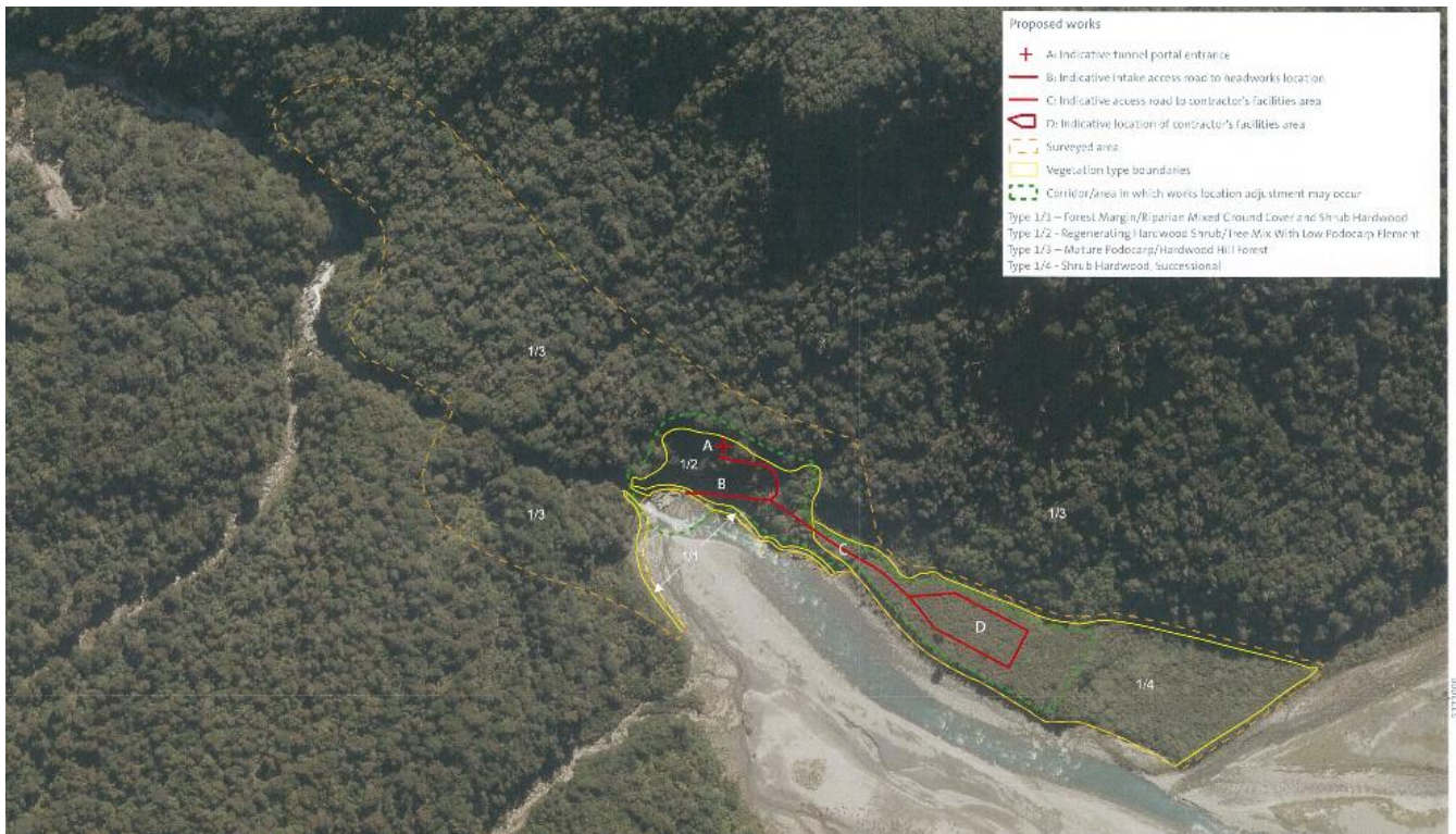
Figure 10 Outlined zones for construction activities Source: Appendix 8 – Ecological Assessment of the Waitaha Hydro Scheme application
