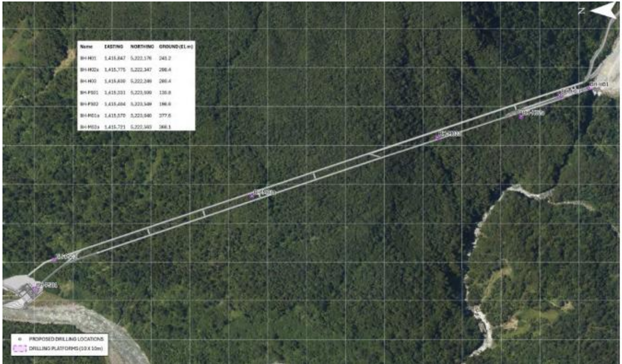
Figure 9 Proposed Geotechnical Investigation Drilling Locations Source: Figure 19, Waitaha Hydro Application Documents
