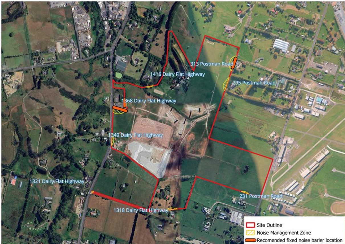
Figure 2 Noise barrier locations
