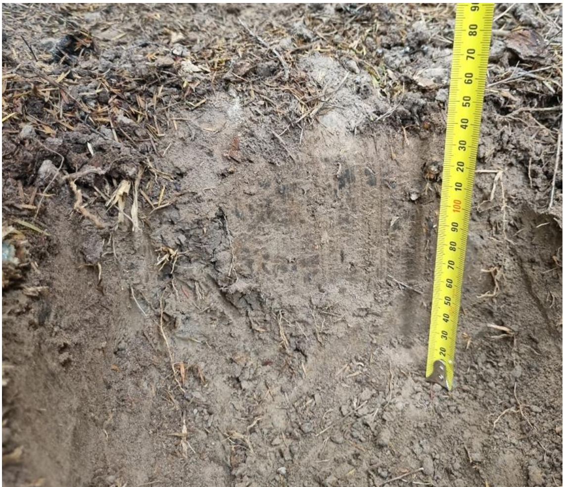
Figure 36. Photograph showing detail of test pit (TP3) in Area 2, showing the hard compacted topsoil
