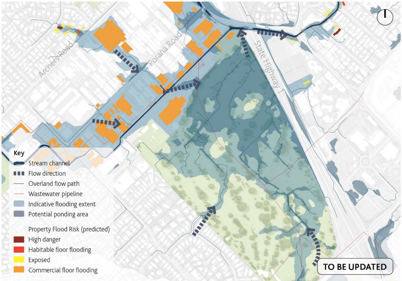
Figure 8: A F Thomas Park flooding
