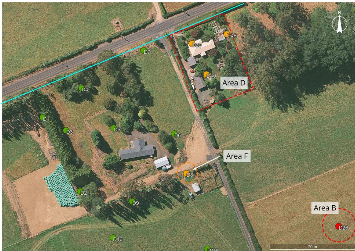
Figure 8: Sampling locations across the northern end of the Site. Red indicates samples that exceed the Commercial/Industrial SCS/SGV, and orange indicates samples above background but below the Commercial/Industrial SCS/SGV. Green indicates samples consistent with predicted background. Areas outlined in red indicate verified HAIL sites, and areas outlined in orange indicate unverified HAIL sites (Google Earth, Image © 2025 Airbus).
