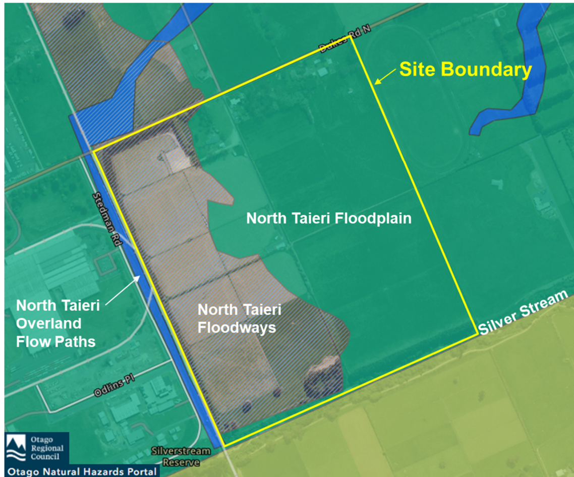
Figure 4. Flood hazard characteristics of the Site area, from Otago Regional Council's Natural Hazards Portal and based on ORC (2015)
