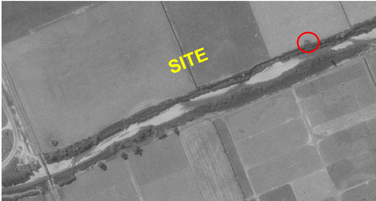
Figure A9. 1985 aerial imagery of Silver Stream (Retrolens), showing first noted occurrence of potential slope instability area (circled in red) near southeastern corner of Site
