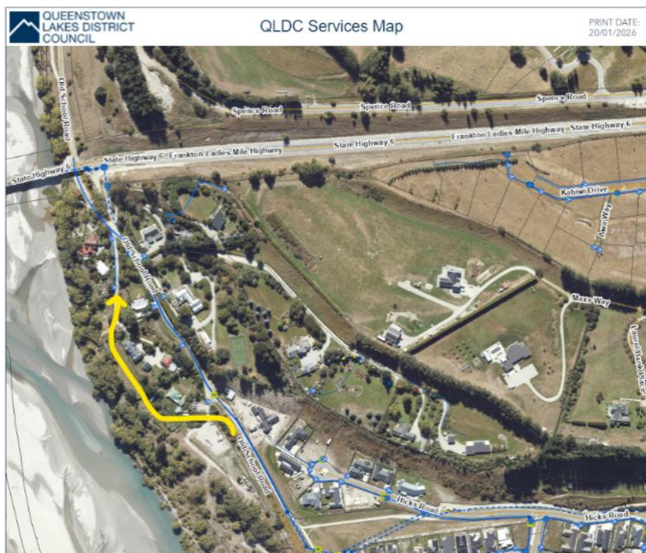
FIGURE 15: YELLOW LINE REPRESENTS PROPOSED ALIGNMENT OF NEW WATER PIPE THROUGH CROWN PARCEL. BLUE LINES REPRESENT EXISTING WATER INFRASTRUCTURE.
