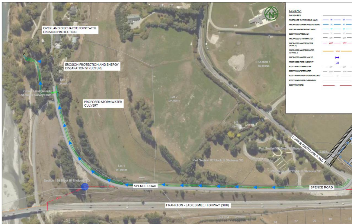
FIGURE 13: PROPOSED EXTERNAL WORKS: STORMWATER DISCHARGE FROM STORM EVENTS GREATER THAN THE 1% AEP EVENT
