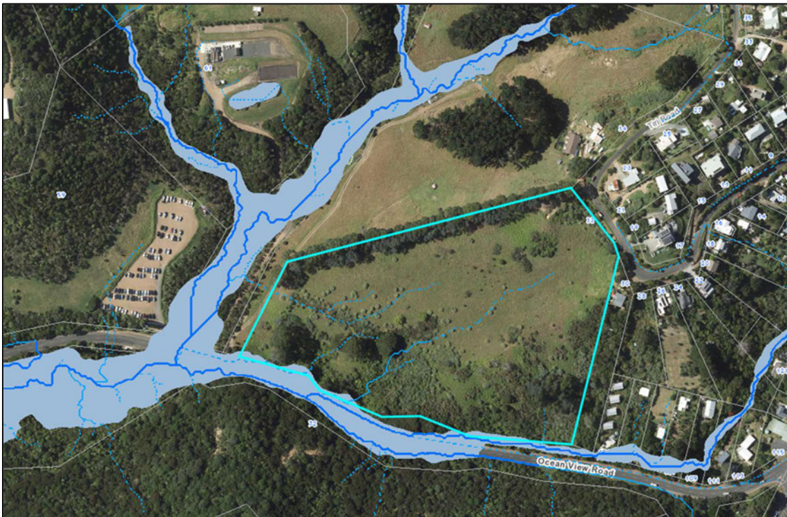
Figure 1: Existing flooding and OLFP around the subject site. Source: AC Geomaps.
