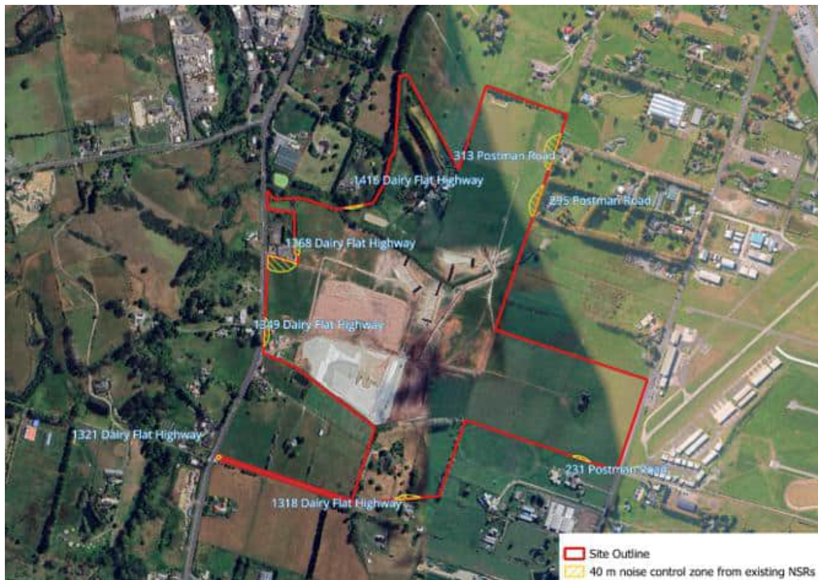
Figure 9 40m construction noise and vibration management zones
