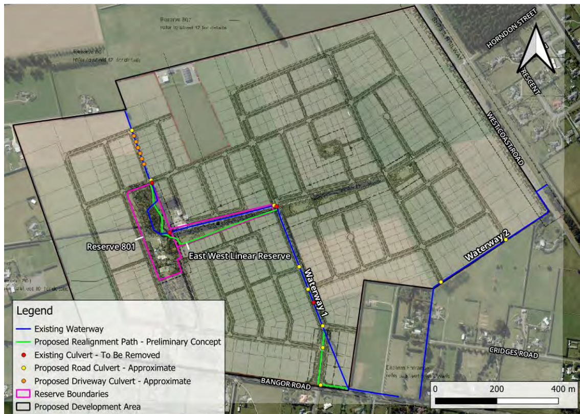
Figure 4 – The proposed realignment and culvert works.
