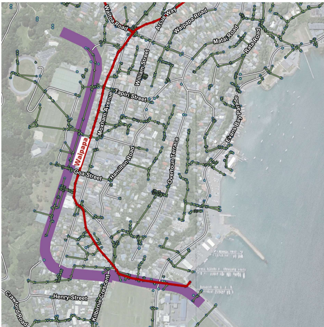
Figure 12 – Waipapa awa and Eastern Connections stormwater systems
