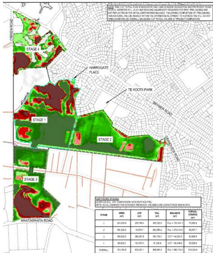
Figure 2: Proposed Cut/Fill Plan
