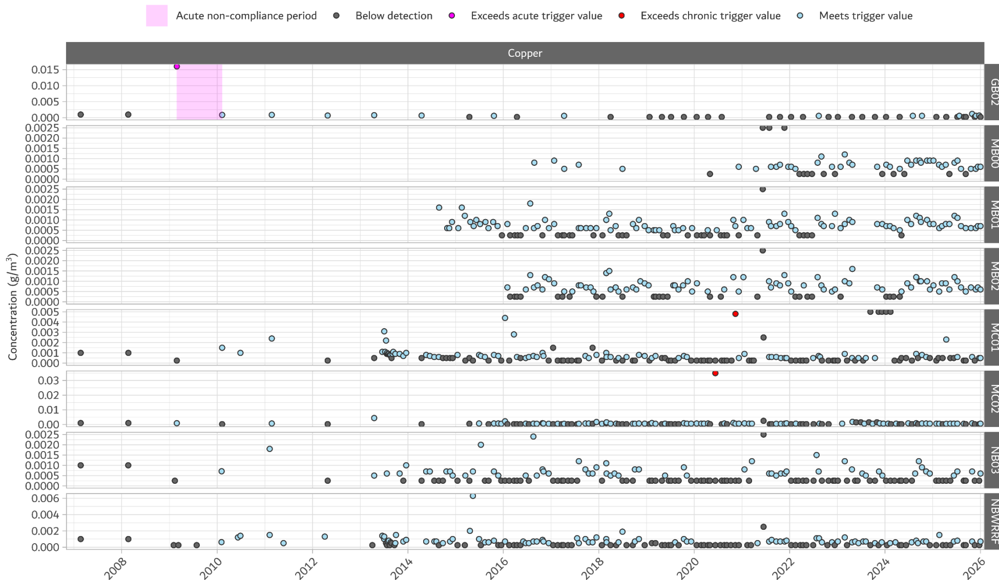
Figure B16. Historical dissolved copper measurements at key compliance sites within the Waikouaiti and Taieri River catchments, assessed against the proposed chronic and acute triggers. Note: scale excludes isolated below detect measurements in 2003 and 2004 at sites GB02, MC01, MC02, and NB03.
