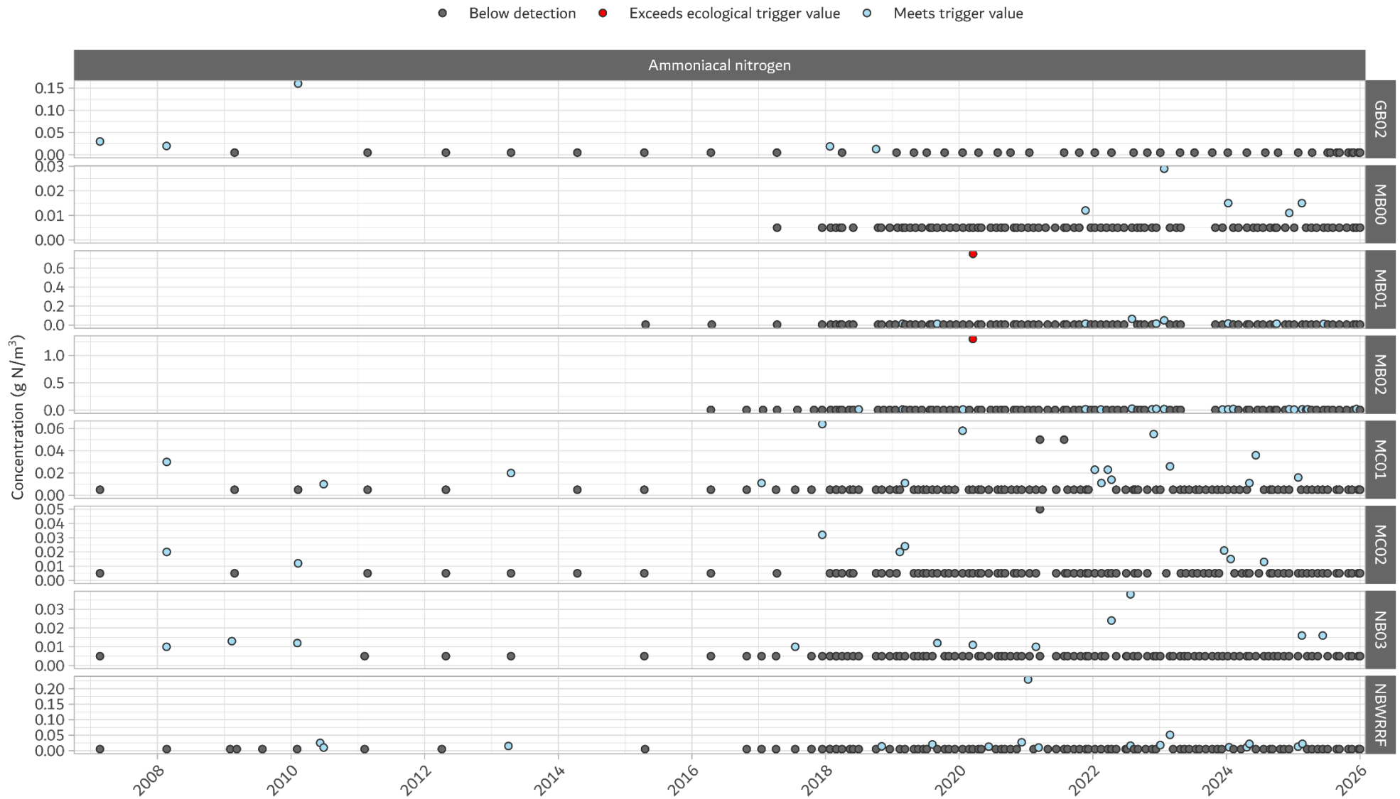
Figure B8. Historical ammoniacal nitrogen measurements at key compliance sites within the Waikouaiti and Taieri River catchments, assessed against the proposed trigger.
