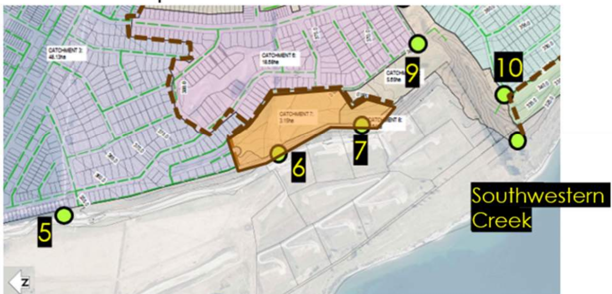
Figure 4-14: Outlets 5, 6 and 7 each drain to an existing culvert under Chief Reko Rd - Pre and Post Development Catchments showing reduction in catchment area
