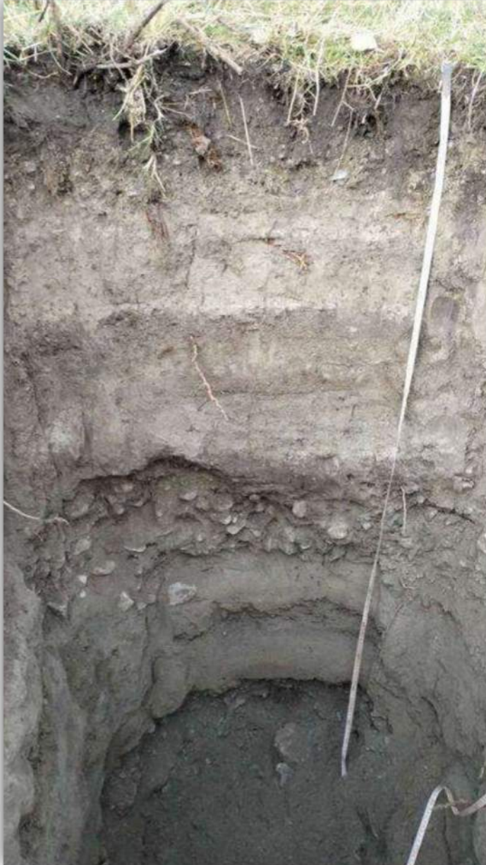
Figure 4-20: Test pit to 1.8m indicating layers of gravels at 1.0m and 1.5m depth between other layers of sand (reference: bore hole HB13/5, Lowe Environmental ImpactSiols Site Investigation, 23 September 2024)
