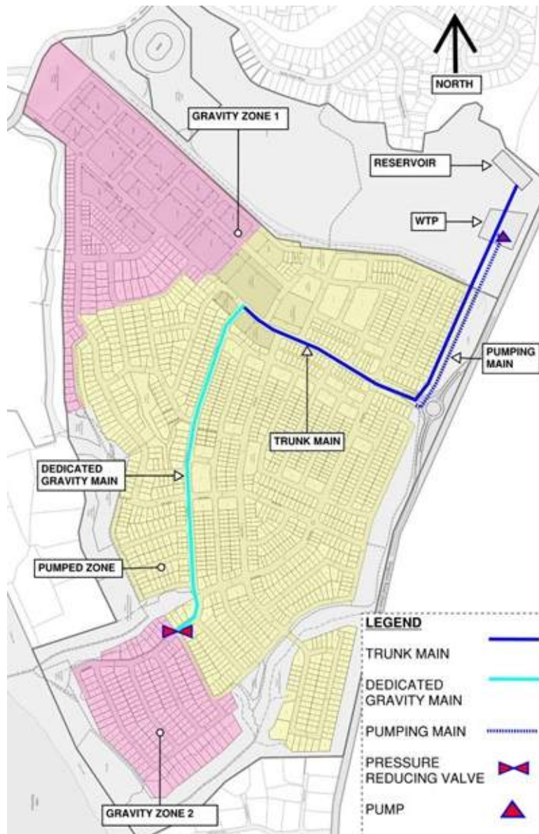
Figure 2-6: Layout of the Boosted Zone, Gravity Zone 1 and Gravity Zone 2
