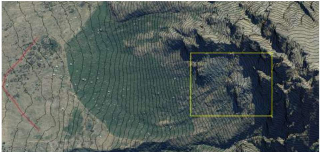
Figure 6-21: Annotated aerial photo showing the location of the inferred maximum extent of cliff collapse debris in red in relation to the Southern Cliffs. The rock fall debris area below some of the rock outcrops is highlighted in the yellow box.
