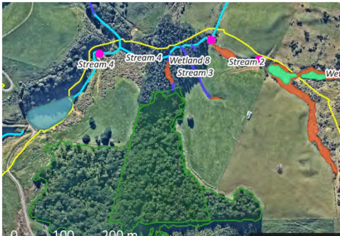
Figure 4 Plan showing the updated pit extent in yellow, allowing the stream / wetland to be retained in-situ
