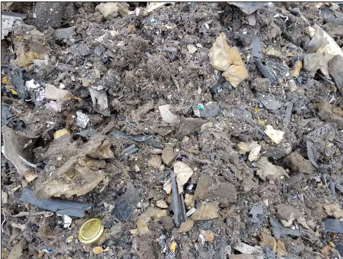
Photograph 2: Close-up of waste output from non-metallic shredder (jar lid ~90 mm diameter for scale)
