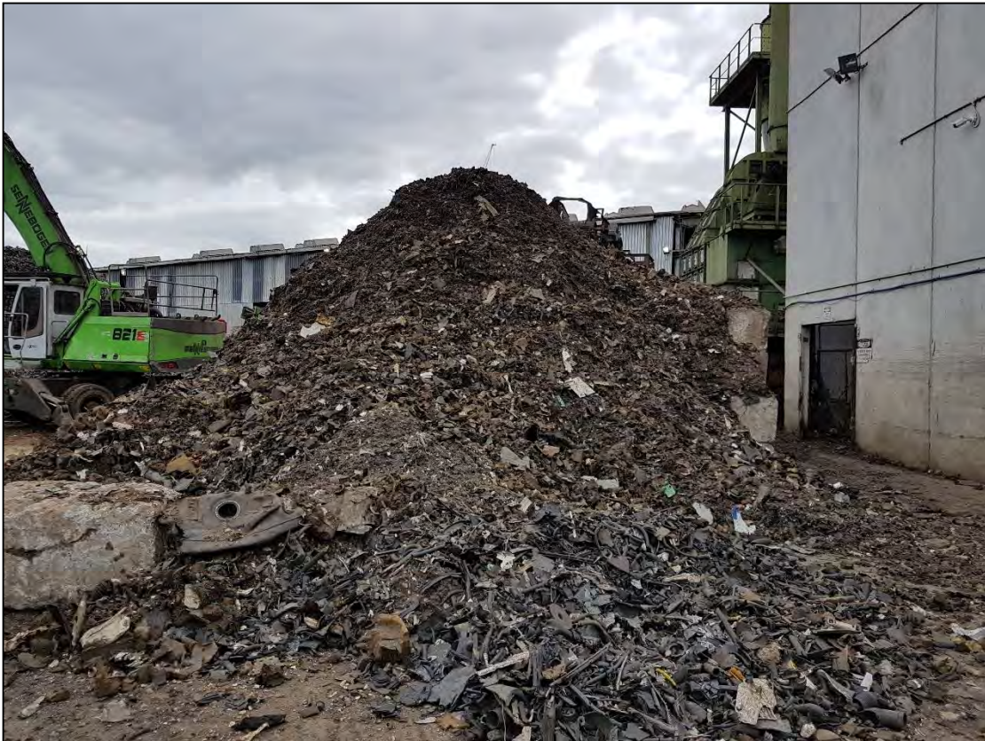
Photograph 1: Overview of waste output from non-metallic shredder
