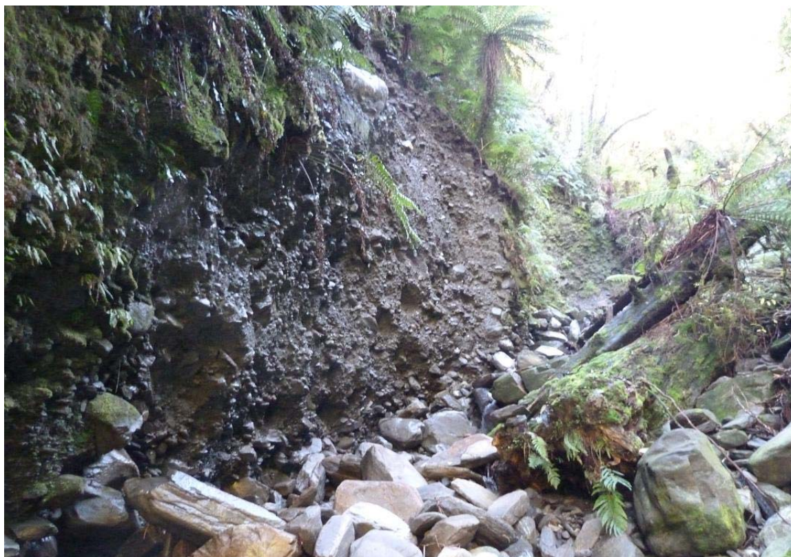
Photograph 2: Post glacial aggradation [pga] gravels exposed in Alpha Creek approximately 100m downstream of the proposed powerhouse.
