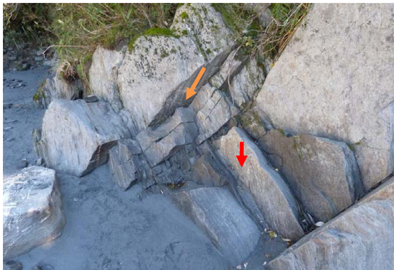
Photograph 5: The most common joint orientation at all the sites [orange arrow], in this case showing up at Whirling Water, where the dips average 50 degrees to the southwest [strike 152 degrees]. The foliation is at approximate right angles to this joint set and is dipping at 80 degrees southeast [red arrow].
