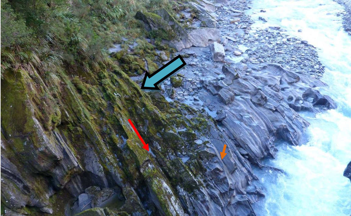
Photograph 7: The bedrock bench on which the intake will be located [river cleaned rock at right of photograph] with the tunnel entry in the direction of the green arrow and at right angles to the bedrock foliation shown by the red arrow. Dominant joint set dip at this location is shown by the orange arrow.
