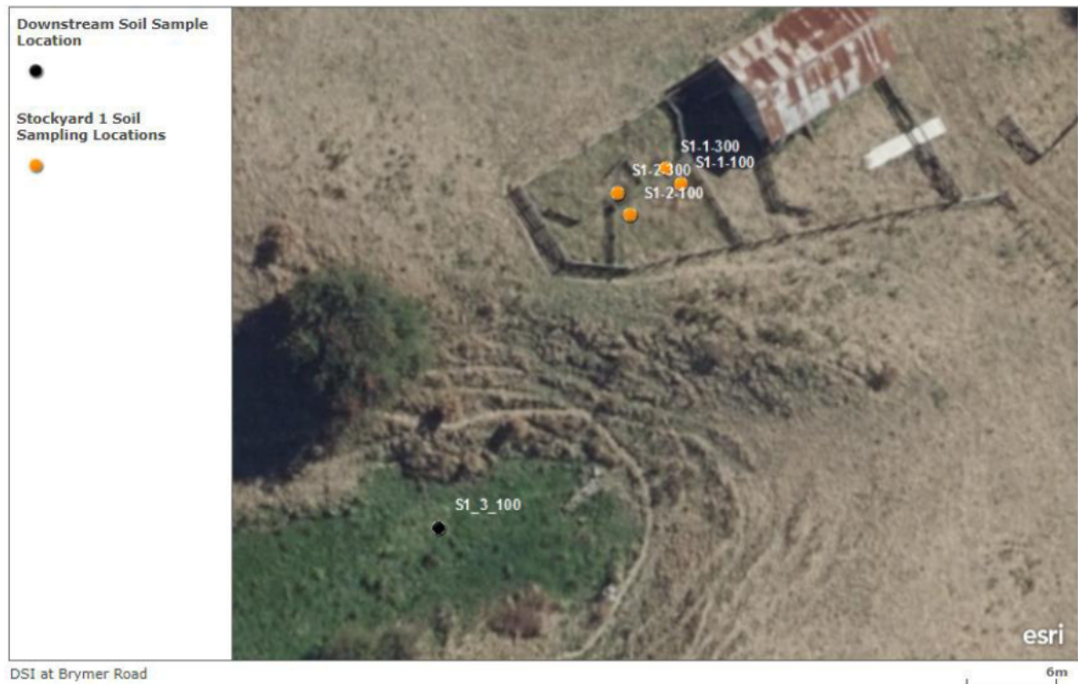
Figure 5.4: Soil sampling locations at Stockyard 1 and downstream. Surface and sub-surface samples are offset for visual display clarity.
