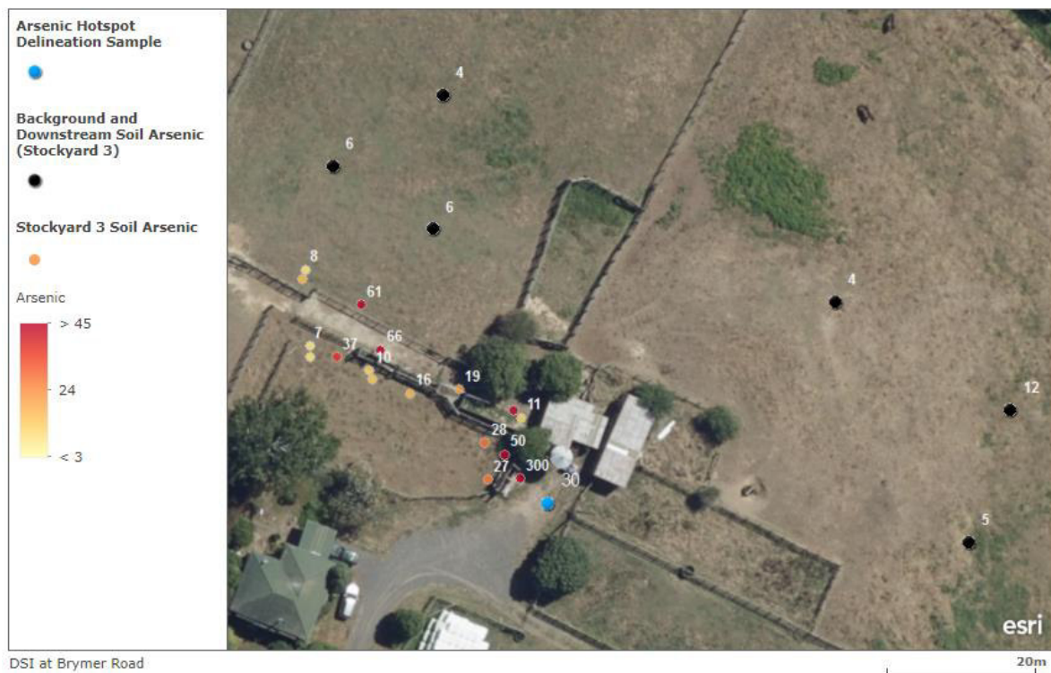
Figure 5.8: Soil arsenic concentrations at Stockyard 3 and downstream / background concentrations. Data for both surface and depth samples are presented and offset for visual display clarity. Numerical values adjacent to sampling locations represents arsenic concentration in mg/kg.
