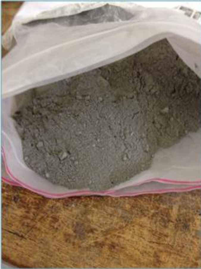
Photograph 2.1: Sediment 1 – TTR. X451. 2 kg. Post-grind tailings. Composite sample.
