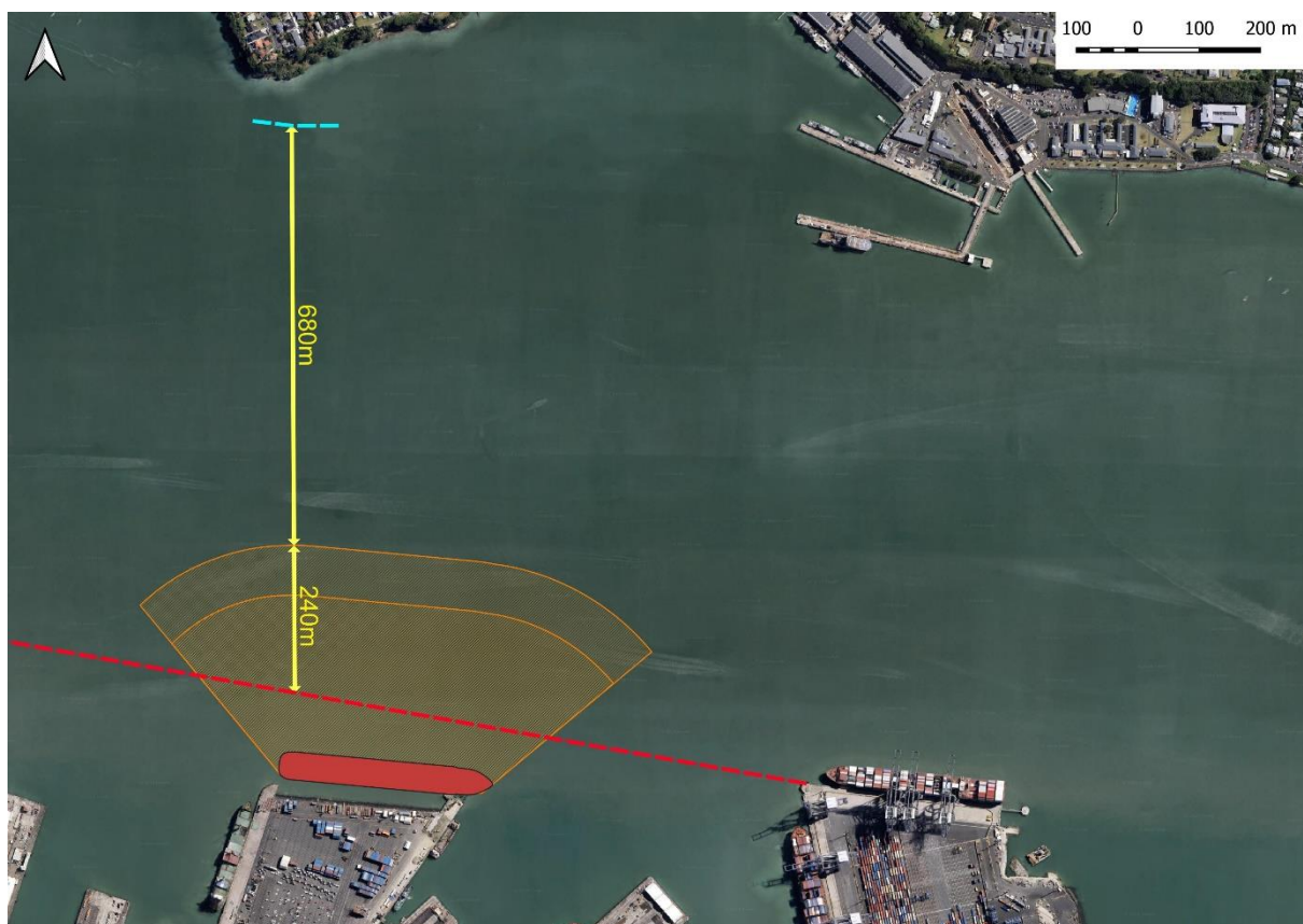
Figure 7-4: Wind shadow of a representative, large cruise ship alongside the proposed Bledisloe North Wharf.
