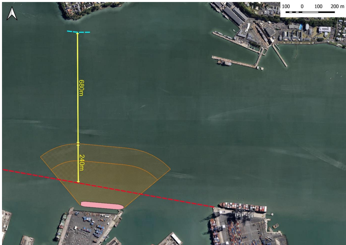
Figure 7-3: Wind shadow of a representative RoRo vessel alongside the new Bledisloe North Wharf.
