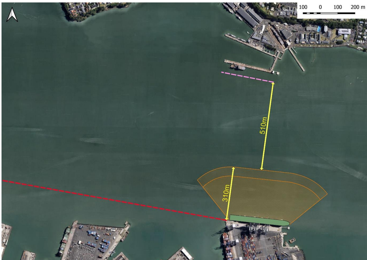
Figure 7-2: Wind shadow of a representative 10,000 TEU container vessel alongside Fergusson North Wharf.
