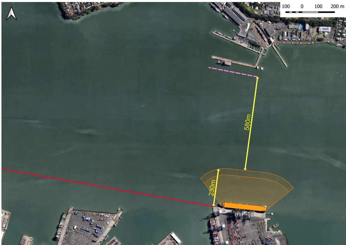
Figure 7-1: Wind shadow of a representative 4,300 TEU container vessel alongside Fergusson North Wharf.
