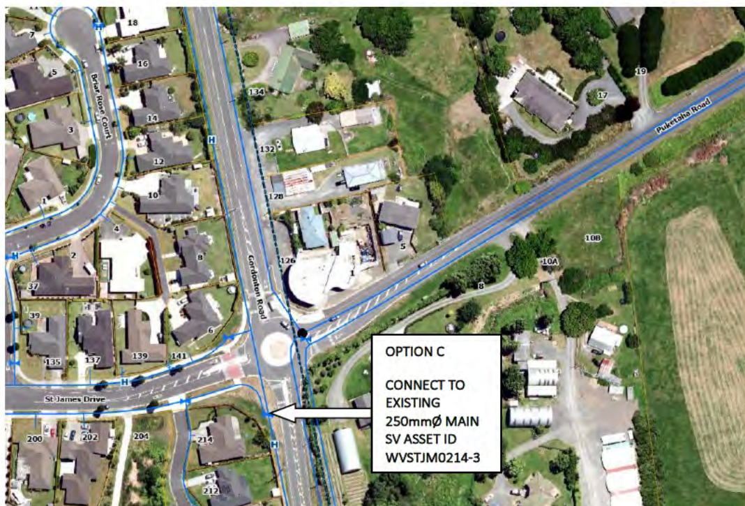
Figure 28 – Existing HCC Water Supply Connection Option C
