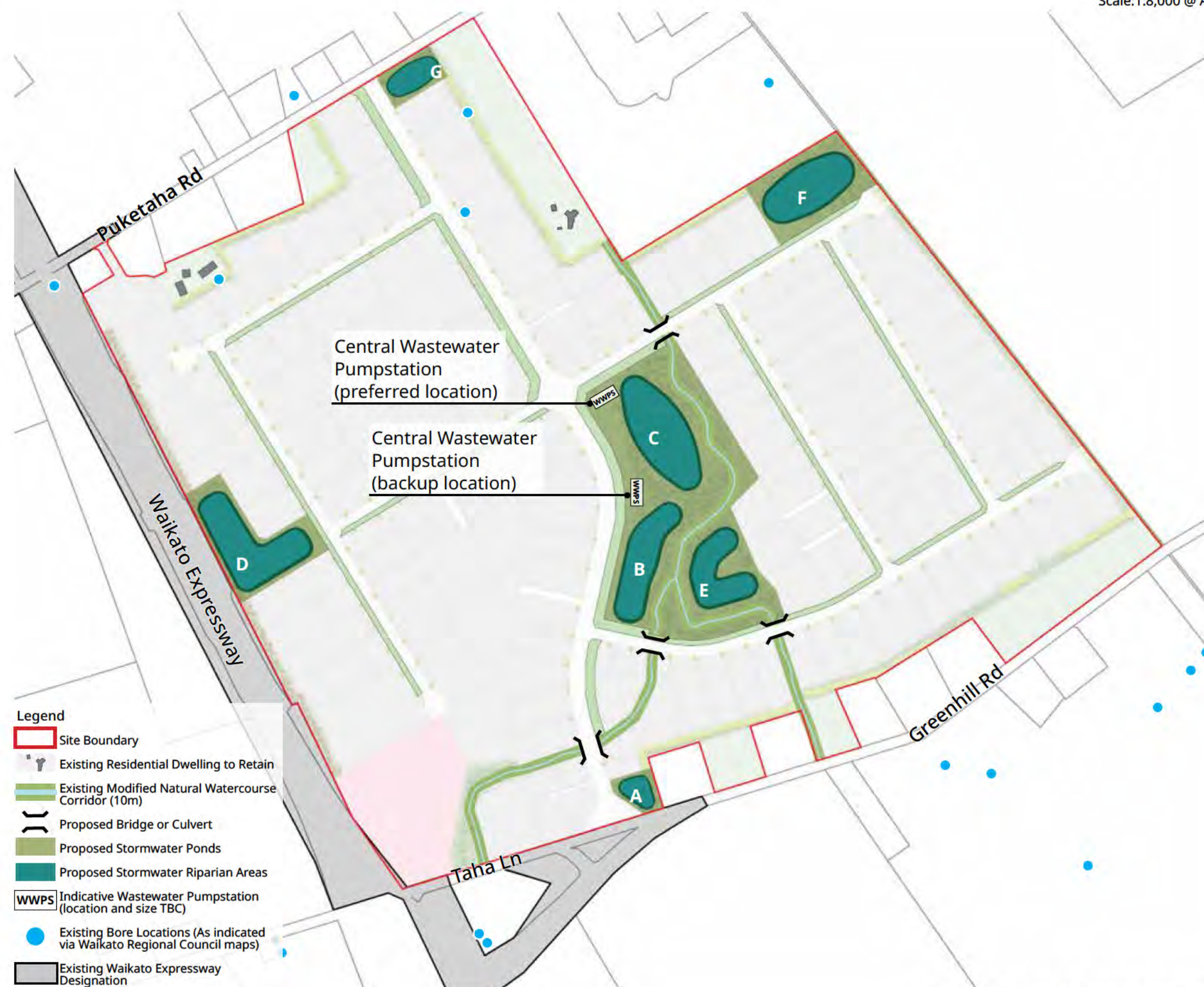
Figure 13 Proposed Water and Wastewater Infrastructure
