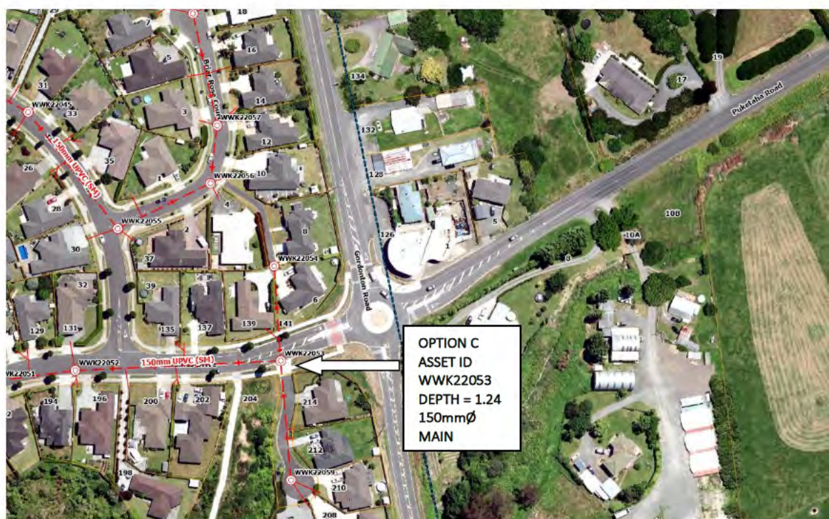
Figure 20 – Existing HCC Wastewater Connection Option C
