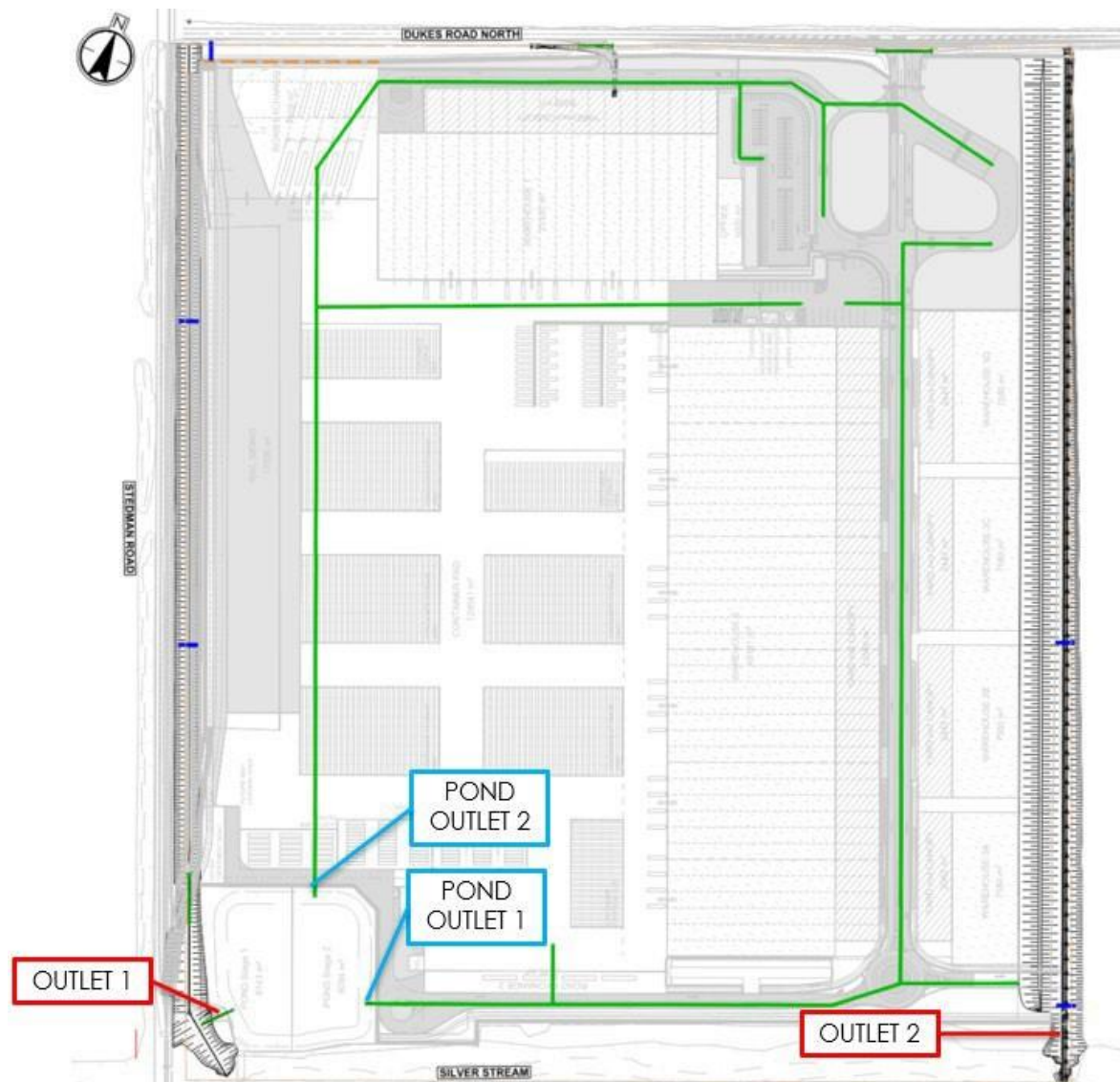
Figure 3: Stormwater treatment and discharge plan (Stantec, 2026). GPT/UPT proposed at Pond Outlet 1 and 2. Outlet 2 conveys 'external' stormwater only.
