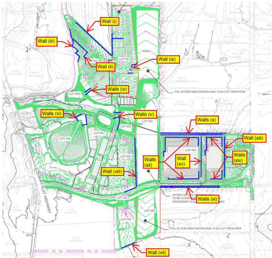
Figure 7-8: Proposed retaining wall locations
