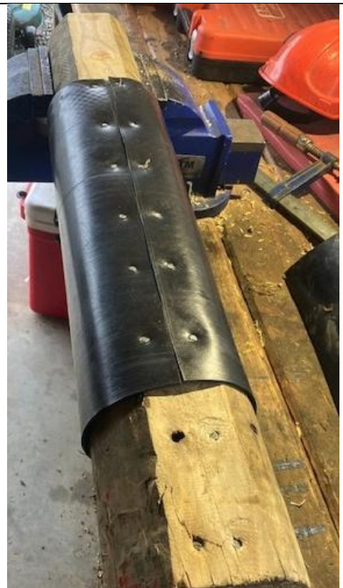
Photograph Appendix H.2: HDPE membrane attached to post.
