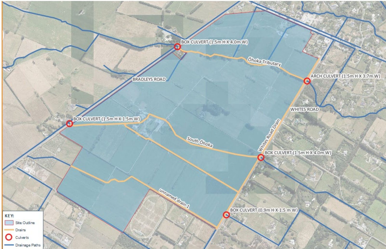
Figure 2: Existing Stormwater infrastructure.
