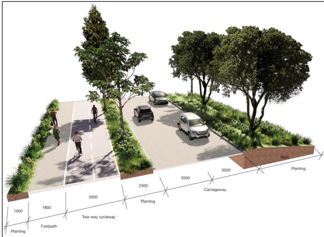
Figure 28: Jack Lachlan Drive Cross Section – Segment B
