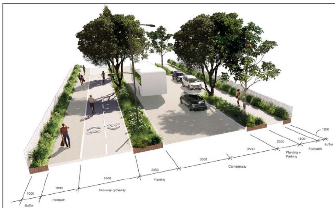
Figure 27: Jack Lachlan Drive Cross Section – Segment A
