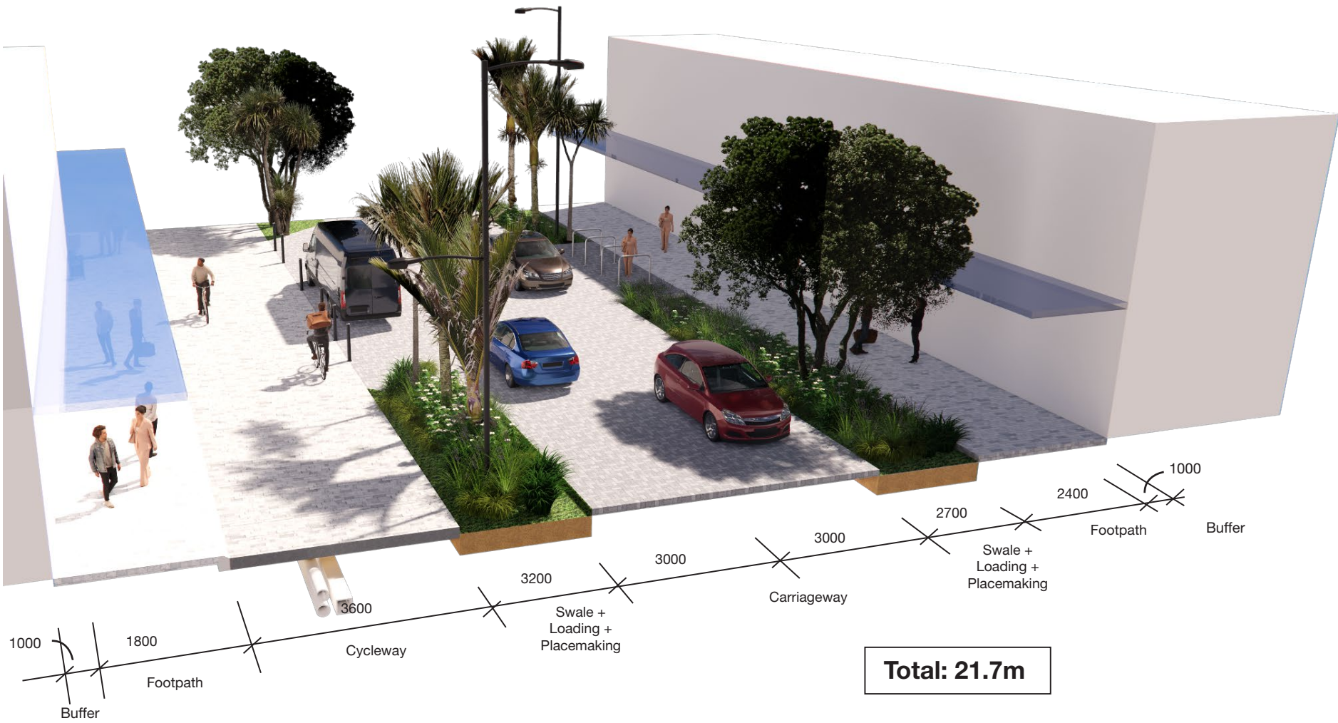
Figure 4. Street Cross-section: Village Centre Secondary Road
