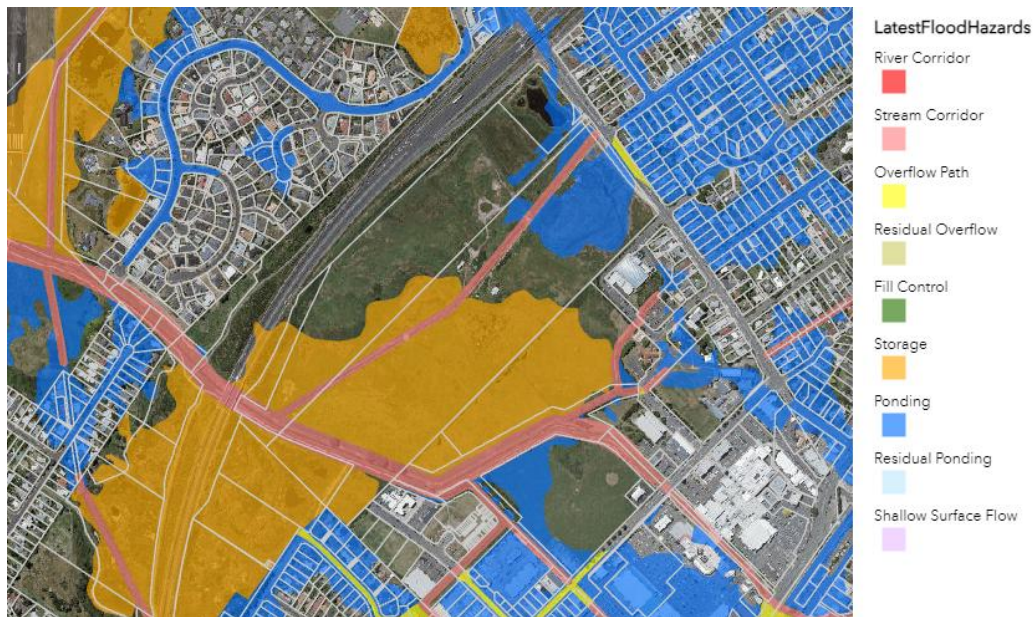
Figure 1. KCDC flood hazard mapping (GIS).
