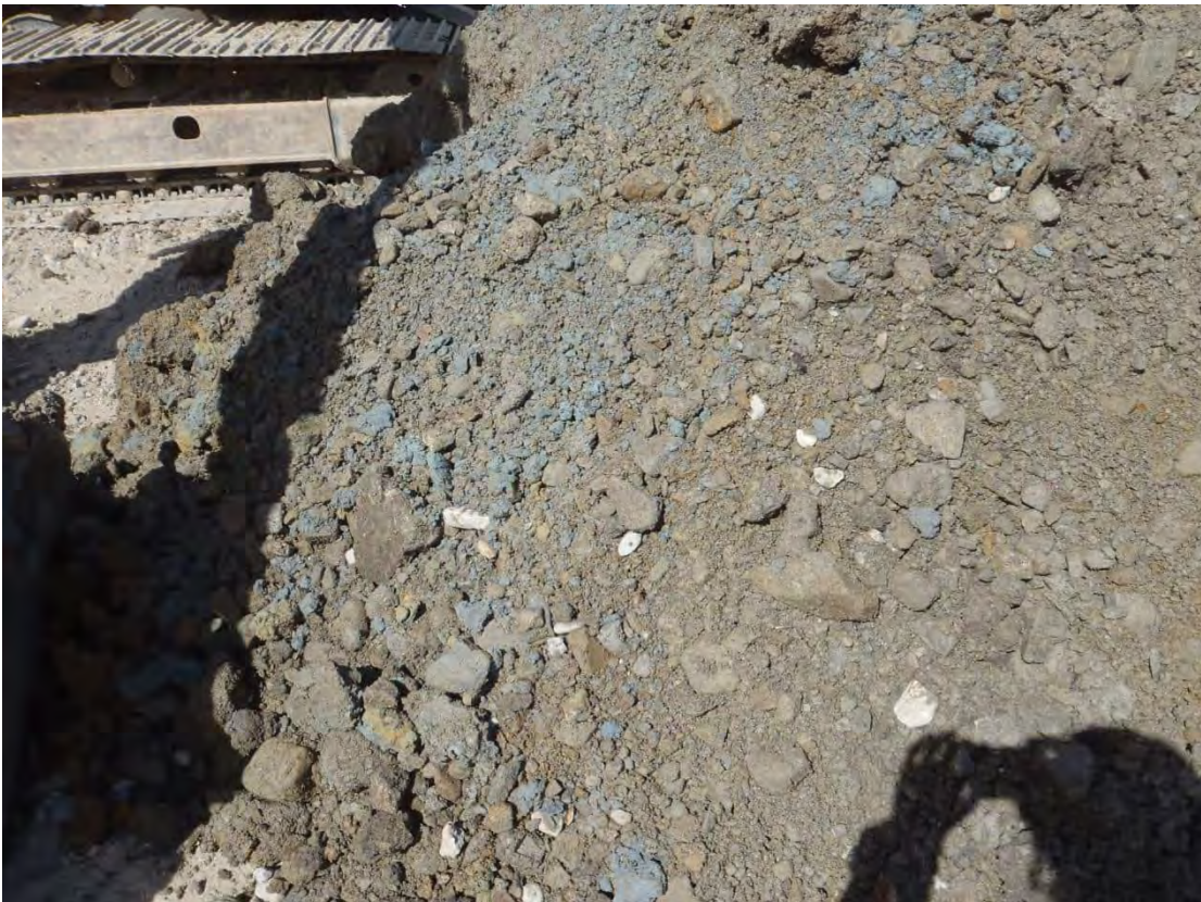
Photograph 4: Spoil from test pit 6, showing blue-grey silty clay from 3.5 m bgl.
