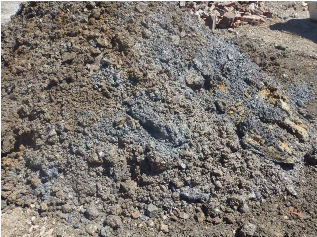
Photograph 14: Spoil from Test pit 14, blue-grey silty clay evident.
