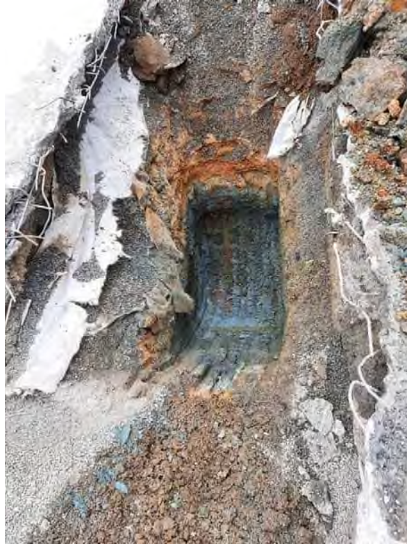
Photograph 7: The photograph shows the location of sample FL01 where stained soils with a hydrocarbon odour were encountered during excavation works.
