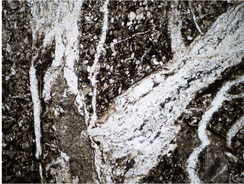
Photo 21: Sample 2606 (BH2B_1144 53.40): Brecciated shear zone (left side) cutting a quartz vein with small prismatic prehnite crystals and other thin quartz-rich veins. Thin (post-shear?) quartz-zeolite veins are present at left and right in siltstone. Field of view = 3.0 mm, plane polarised light.
