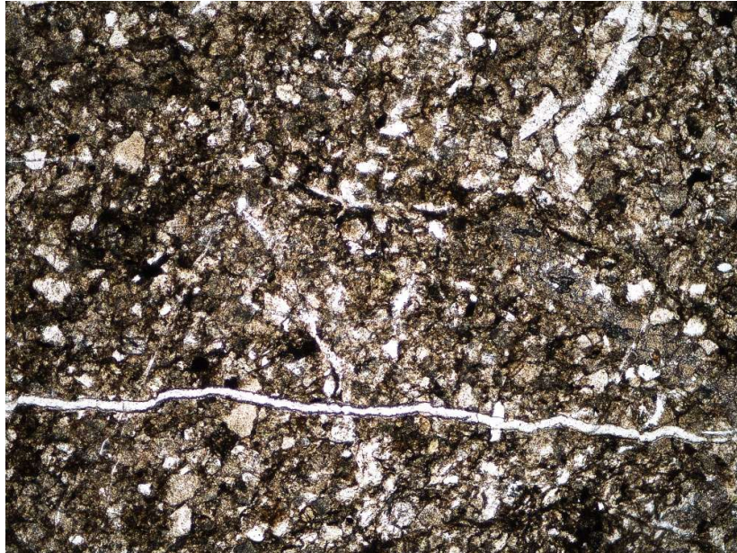
Photo 15: Sample 2603 (BH2B_1144 40.50): Siltstone, cut by a thin continuous calcite vein (bottom) and fragmented quartz (top right) and prehnite (centre right) veins. Field of view = 3.0 mm, plane polarised light.
