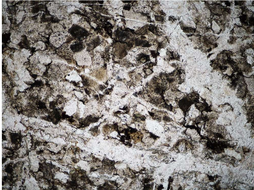
Photo 13: Sample 2602 (BH2B_1144 33.17): Sandstone, cut by quartz-rich veins, with minor calcite in some (centre left). Field of view = 3.0 mm, plane polarised light.
