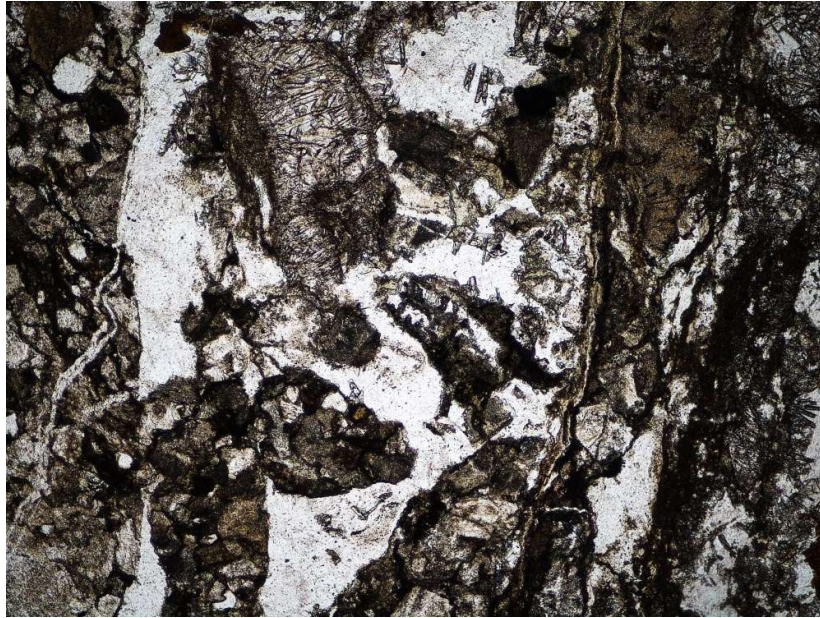
Photo 23: Sample 2609 (BH2B_1117 22.35): Breccia, comprising elongate sandstone and vein fragments in a quartz-rich matrix. Field of view = 3.0 mm, plane polarised light.
