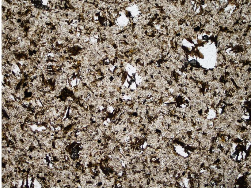
Photo 7: Sample 2719 (BH2B_1157 51.70-52.05): K-feldspar and plagioclase phenocrysts in fine grained quartz, plagioclase, K-feldspar, altered mafic minerals and granular opaque minerals. Field of view = 3.0 mm, plane polarised light.
