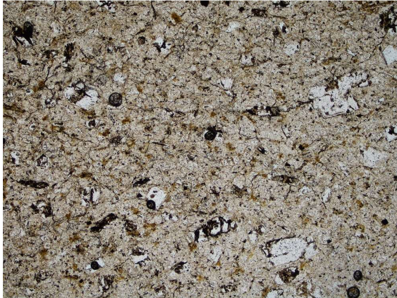
Photo 3: Sample 2717 (BH2B_1157 31.10-31.25): Small K-feldspar phenocrysts surrounded by fine quartz, plagioclase, K-feldspar, altered mafic minerals and granular opaque minerals. Field of view = 3.0 mm, plane polarised light.
