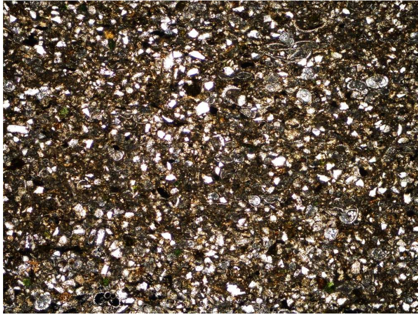
Photo 7: Sample 2597 (BH2B_1105 38.25): Calcareous siltstone, containing rounded foraminifera tests and subangular detrital crystals in a matrix of fine calcite and clay. Field of view = 3.0 mm, plane polarised light.
