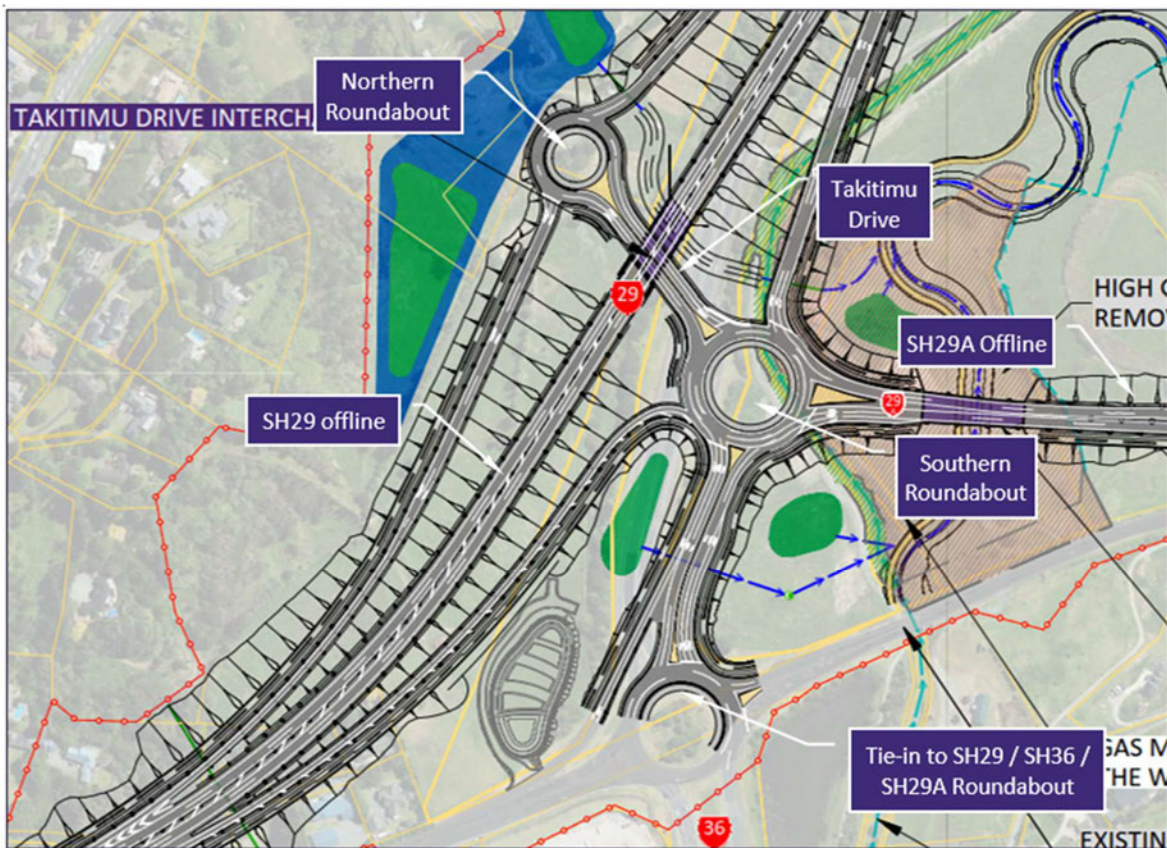
Figure 4.17 – SH29 offline - SH29 / SH36 Roundabout Road Tie-in
