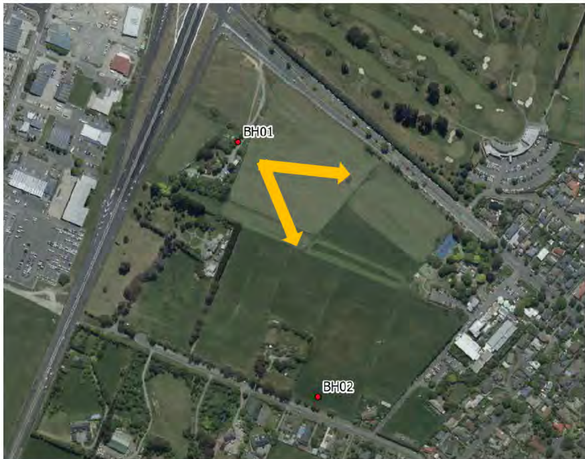
Figure 3. Groundwater Flow Direction (orange arrow)
