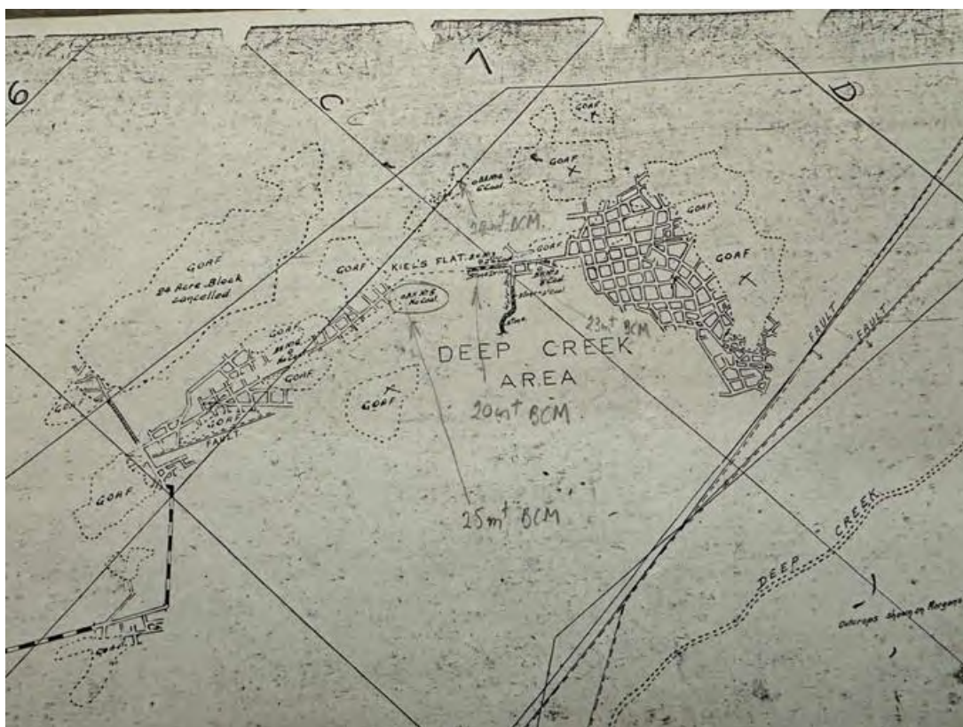
Figure 34. Detail from plan of Main Lease Iron Bridge (Jul 1945) State Coal Mines Survey Office, Granity, showing the Taipo Mine workings in the Deep Creek area (Bathurst Archives S00014403 / 04-01-012)
